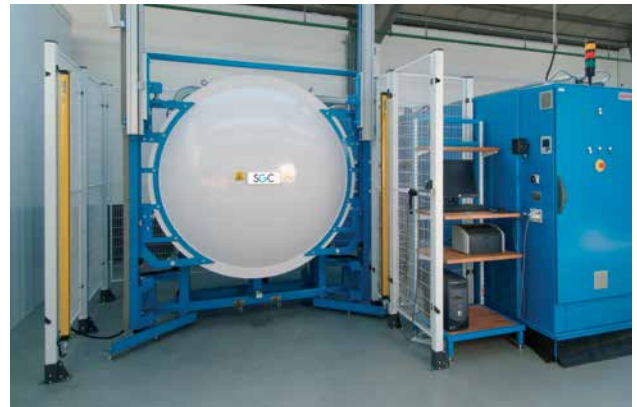
SF 6 filling and sealing station
