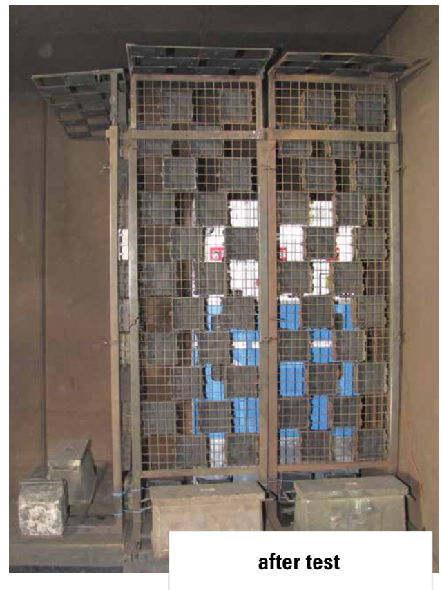
The various tests were always in accordance with IAC specifications by the standard IEC 62271-200
