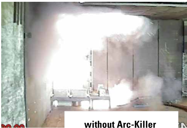
KEMA type tested according to IAC: B, FLR 20 kA 1 s. This solution is patented.
