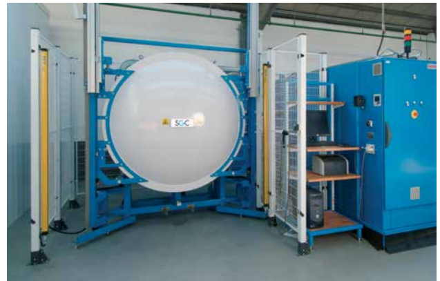
SF 6 filling and sealing station
