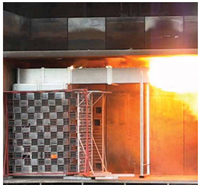
Internal arc fault test, 31.5kA/1s
