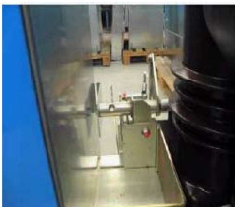
Photo 10: drilling in main axis of arc-killer
