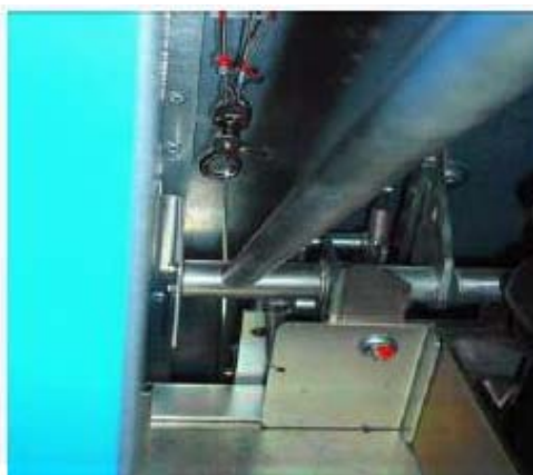
Photo 11: Operating handle in drilling space
