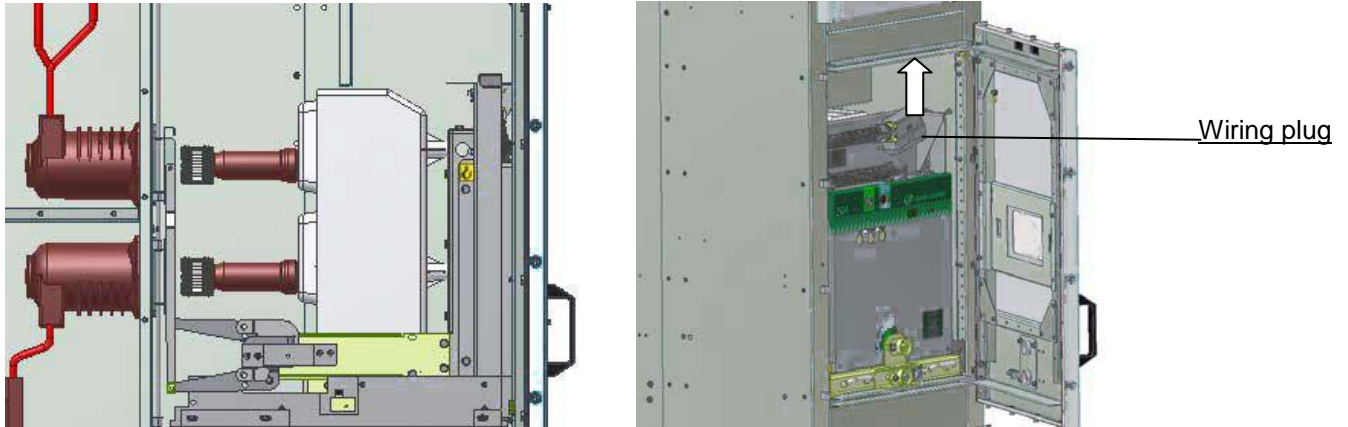
Figure 49 ISMD in test/disconnected position
