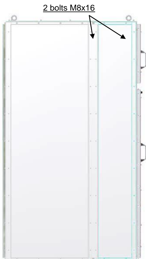
Figure 39 Installation of the front lateral wall. Bolt M8x12 and washer, 11 pcs Bolt M8x16 and washer, 2 pcs
