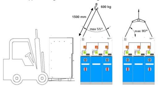
In order to safely and securely lift the unit, use the provided **lifting eyebolts**. Secure the slings or rocker arms tightly to all four lifting eyebolts before moving the unit into its final position.
