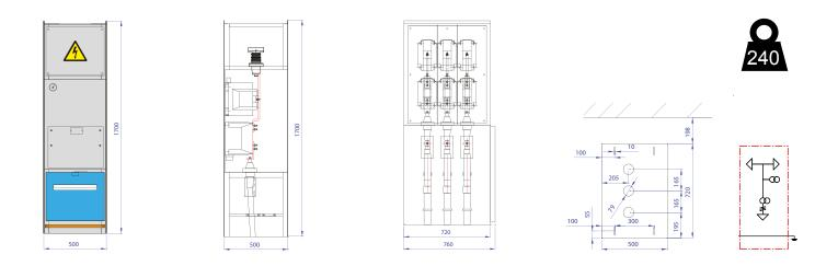
Possible connections: Bottom in - top out, bottom in - top left out, bottom in - top right out
