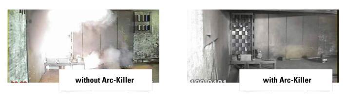
SGC nv SwitchGear Company's patented SV-25 Arc-Killer takes **safety to a new level**. Not just the operator and the environment are shielded from harm, but the super-swift arc extinguishing system allows cubicles to be back in operation very quickly in case of an internal fault. What's more, **the arc-killer's improved security features place less strict demands on the installation room**. As such, the Arc-Killer couples security and operational safety, with flexible room demands.
