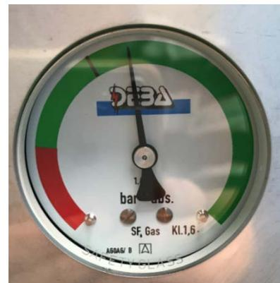
Figure 15: Gas pressure monitor
