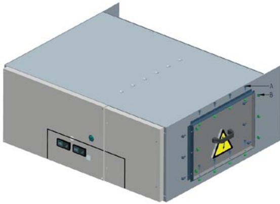
Figure 5: Disassembly of the access hatch
