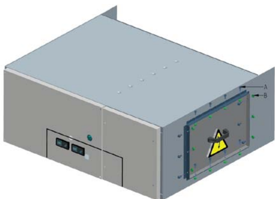
Figure 14: Disassembly of the access hatch
